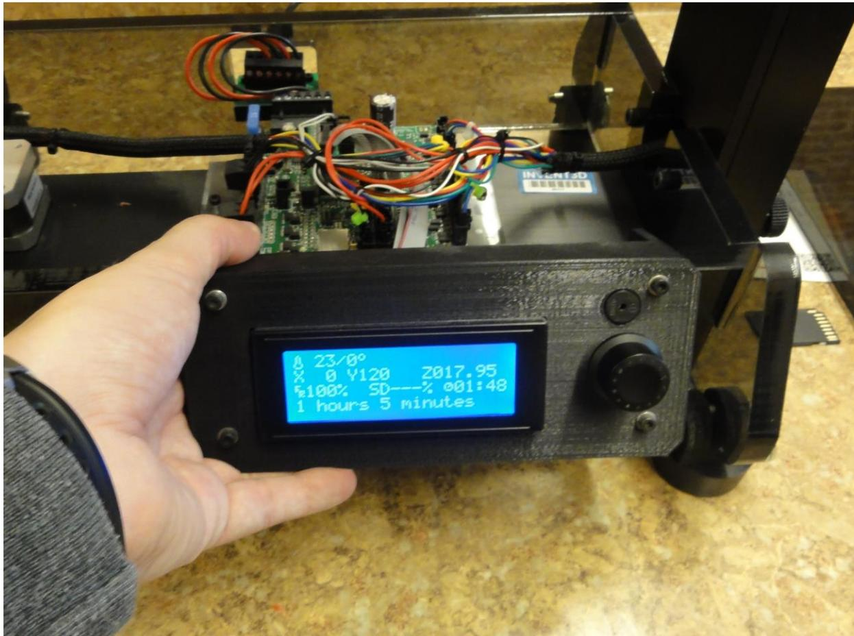
**Step 2** – Grab the LCD display and lift it up and out of the front plate. After doing so, set the LCD face down on the table.
