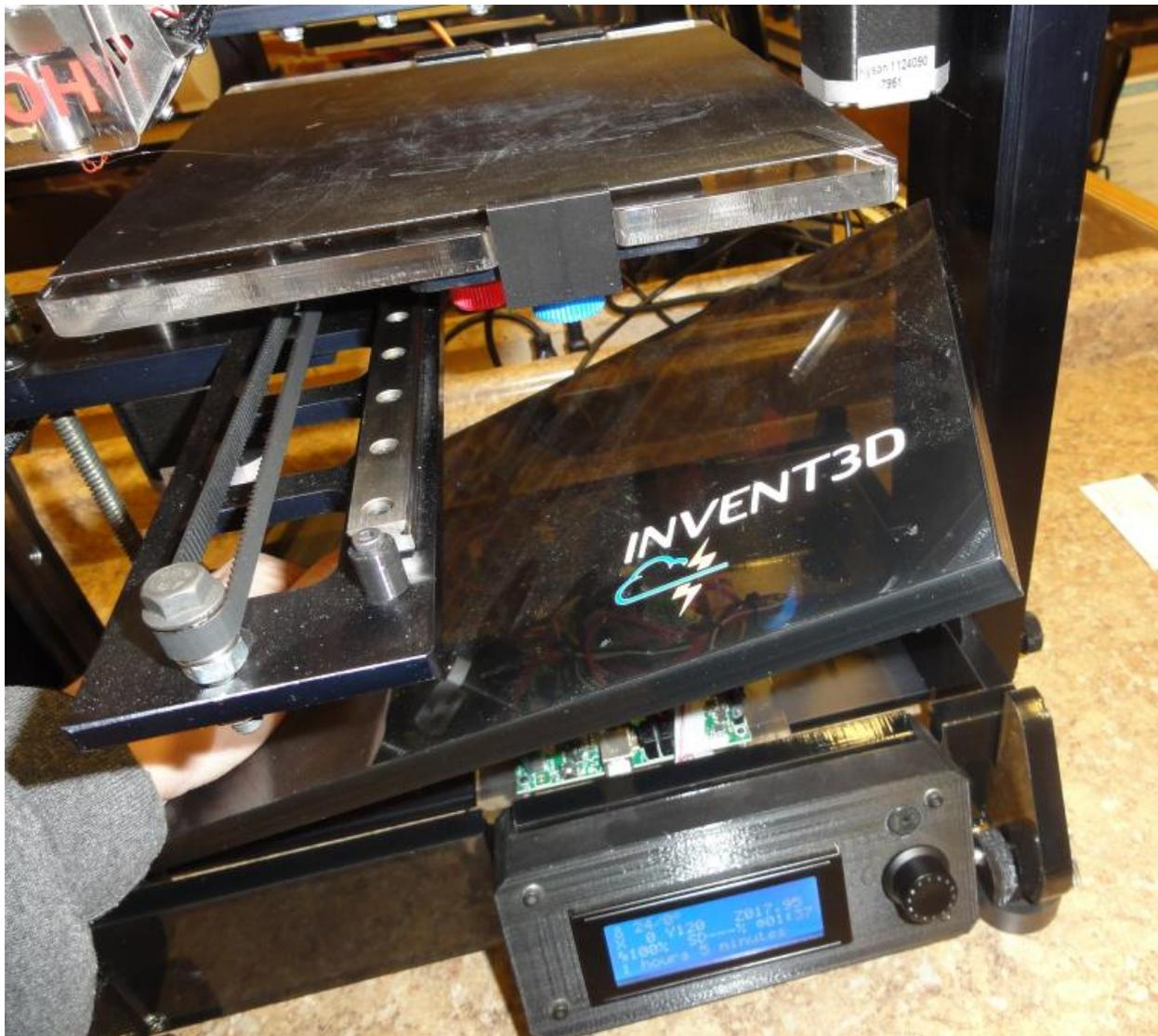
**Step 1** – As shown above, you need to remove the top plate. With the print board positioned near the top of the printer, lift the right side of the top plate up and then swing the right side of the top plate
